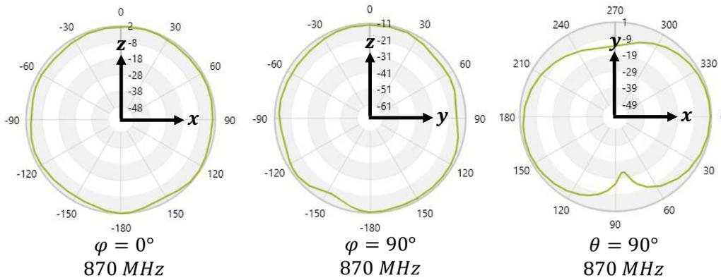
Figure 8: EP112 870 MHz radiation pattern
