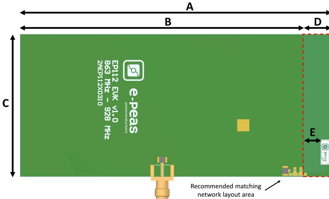
Figure 5: EP112 863-928 MHz EVK dimensions (drawing)
