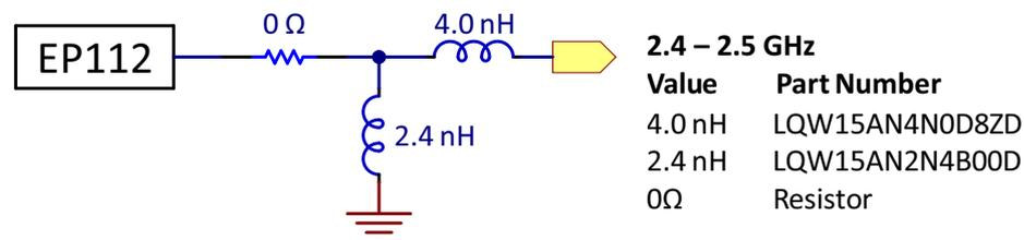
Figure 3: matching network example for 2.4-2.5 GHz frequency range (as on 2540 MHz EVK)
