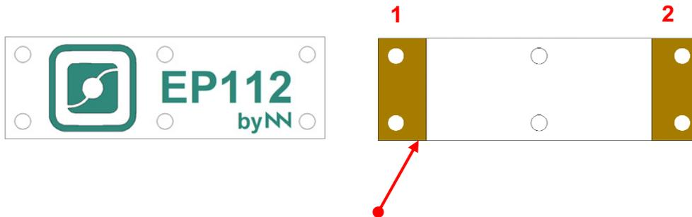
**Feed Pad (1):** The 2 pads are fully symmetrical. Once the feeding pad is selected (1), the other pad (2) will become a mounting pad. Align the feeding pad with the feeding line on the PCB.
