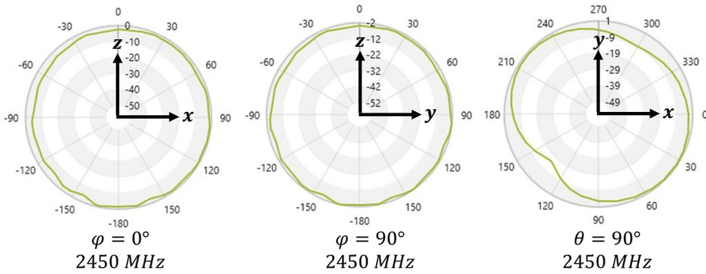
Figure 12: EP112 2400 - 2500 MHz radiation pattern
