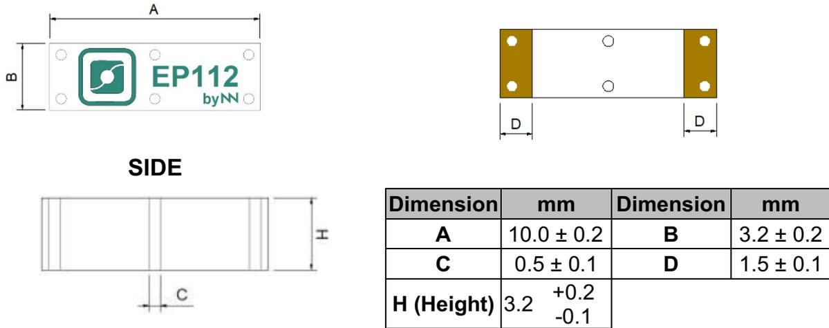
Figure 13: mechanical drawing
