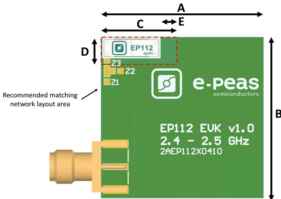
Figure 9: EP112 2.4-2.5 GHz EVK dimensions (drawing)
