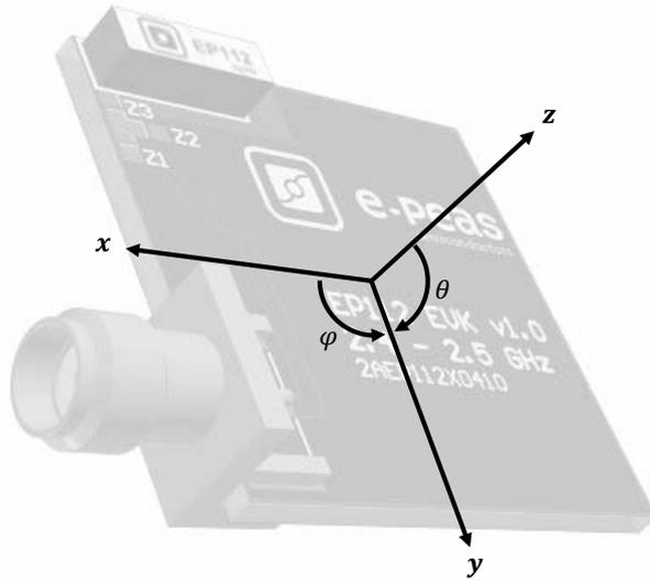
Figure 11: 2450 MHz radiation pattern coordinates
