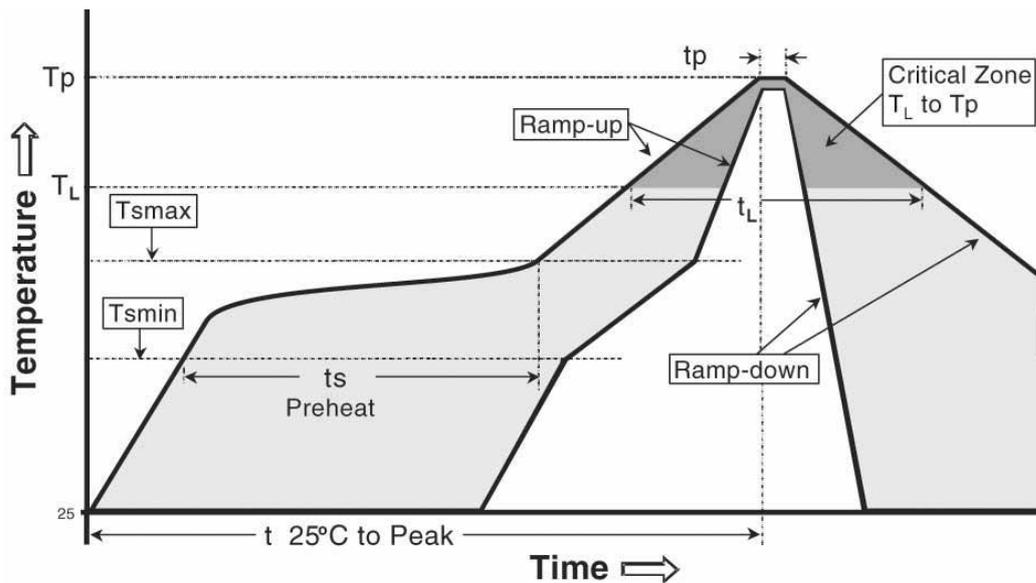
Figure 17: temperature profile for soldering
