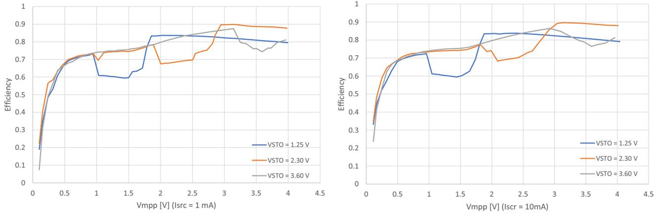
Figure 2: DCDC Efficiency from SRC to STO for 1 mA and 10 mA in Low Power Mode
