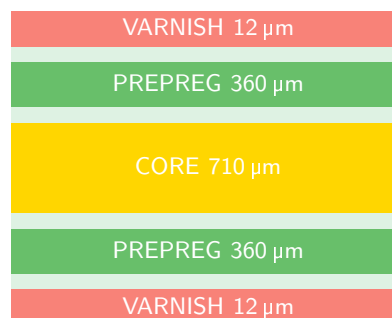
Figure 26: Recommended PCB stackup
