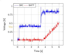
Figure 6: AEM10941 behaviour during cold start
