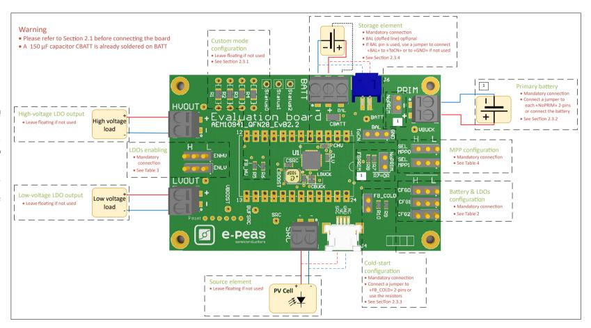
Figure 1: Connection diagram
