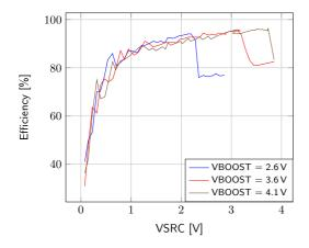
Figure 8: Boost efficiency for ISRC = 1 mA
