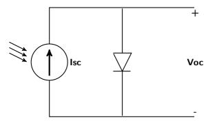
Figure 9: PV cell first order model
